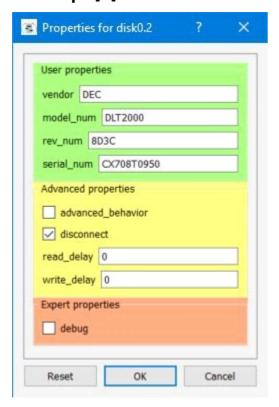
Specific tape drive information can be defined for emulated tapes under Avanti. This is useful to support older operating systems, less common tape drives, or non-DEC tape drives.
