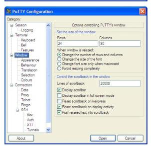
Starting with a default PuTTY configuration, the settings shown below are typically used to access Tru64 UNIX on Avanti virtual Alpha systems via serial or telnet connections:
