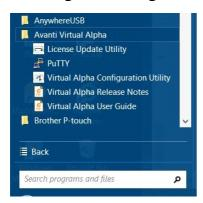
The Avanti Configuration Utility is launched from Start> All Programs> Avanti Virtual Alpha> Virtual Alpha Configuration Utility.
